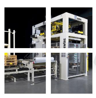
This series of automatic palletizers lets you overlap bags on the same layer. The bag handling principle employed by this machine makes it suitable for the most difficult products.
